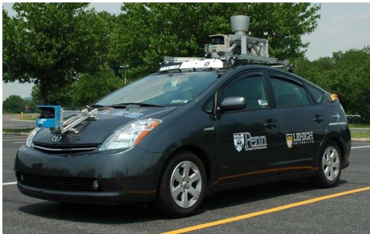
Figure 1: Little Ben is a Toyota Prius hybrid vehicle modified for drive-by-wire operation with an onboard array of sensors and computers.
